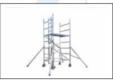
**Step 12** Fit stabilizers ASAP to increase the base dimension. Position the stabilizer so that the foot pads are approximately equidistant from other at 45° for maximum stability.
