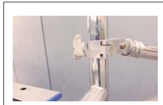
STEP-10 Fit stabilizer ASAP to increase the base dimension, position the stabilizer so that the foot pads area approximately equidistant from other at 45 degree for maximum stability.
